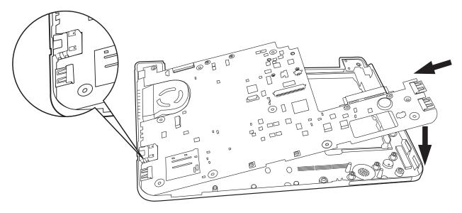
Figure 4.24 Aligning the motherboard connectors
