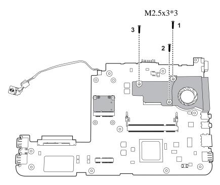
Figure 4.26 Removing the Thermal Fan Module
