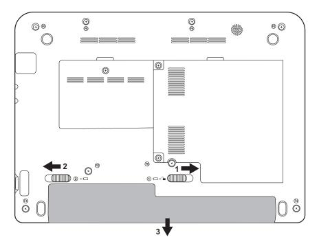
Figure 4.1 Removing the Battery Pack
