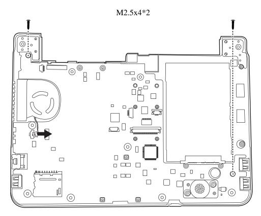
Figure 4.20 Removing the motherboard from logic lower assembly
