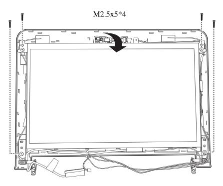
Figure 4.31 Removing the screws from the LCD module
