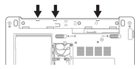
Figure 4.9 Detaching three hinge cap hooks
