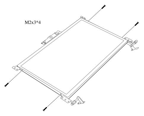
Figure 4.32 Removing the LCD Hinge Assembly
