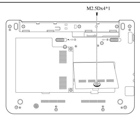
Figure 4.5 Removing the RAM door
