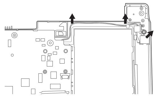
Figure 4.22 Removing the DC IN connector and cable
