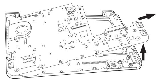
Figure 4.23 Picking up the motherboard
