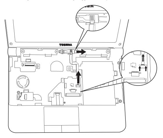
Figure 4.12 Removing the Power Board
