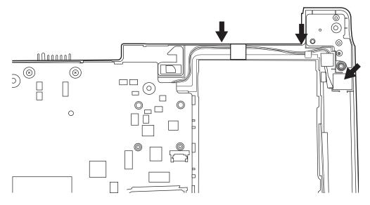
Figure 4.25 Installing the DC IN connector
