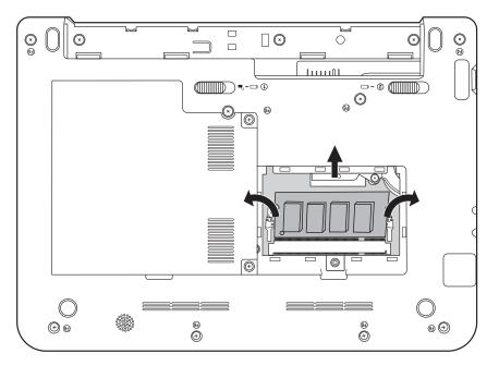
Figure 4.6 Removing the RAM from the laptop
