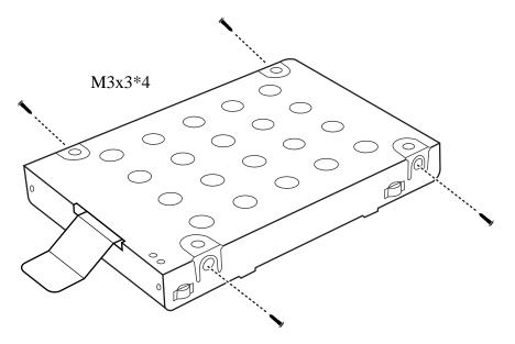
Figure 4.4 Removing the HDD plate
