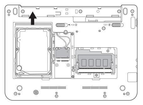
Figure 4.3 Removing the HDD from the HDD bay
