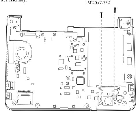
Figure 4.18 Removing the speaker
