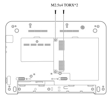
Figure 4.2 Removing the HDD door
