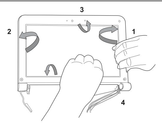
Figure 4.29 Removing the bezel from the hinge wall
