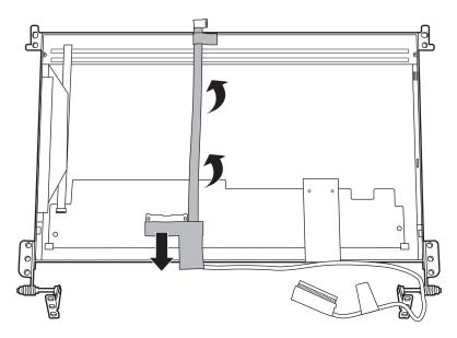
Figure 4.34 Removing the LVDS cable from the LCD module
