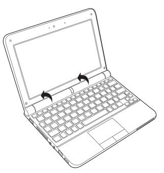
Figure 4.10 Removing the Hinge Cover
