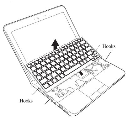
Figure 4.11 Removing the keyboard
