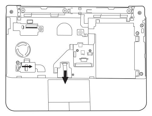
Figure 4.17 Detaching the cables from under the keyboard
