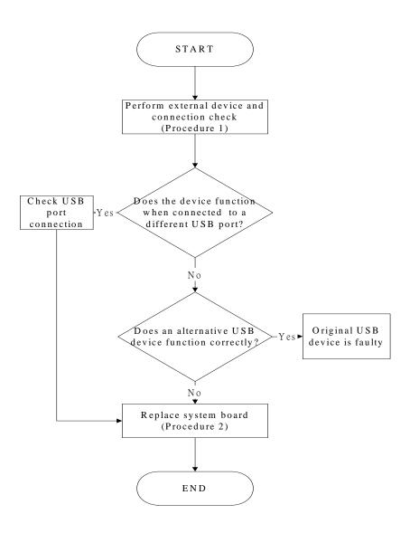
Figure 2-5 External USB device troubleshooting process
