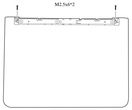
Figure 4.15 Removing the first pair of screws from the hinge saddle
