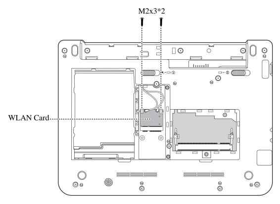
Figure 4.7 Removing the WLAN card
