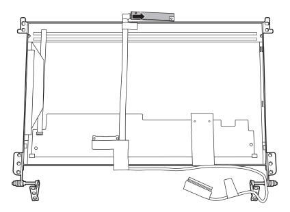
Figure 4.33 Removing the Camera from the LCD panel
