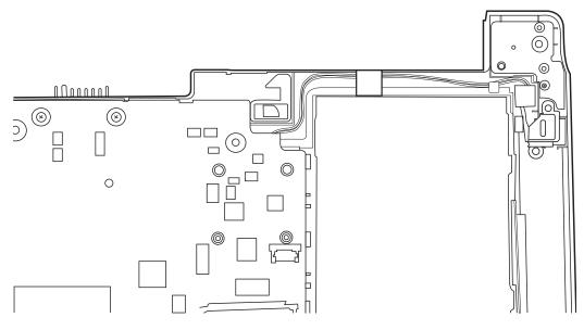
Figure 4.21 Removing the DC IN plate
