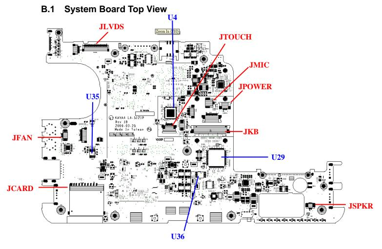
Figure B-1 System Board Layout (Top)
