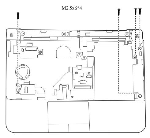
Figure 4.13 Removing three screws from under the keyboard
