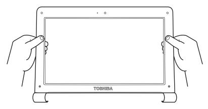
Figure 4.30 Removing the bezel from the display assembly
